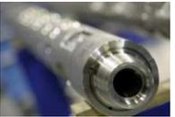
The collars produced by Schoeller-Bleckmann are used as high-tech housings for special logging instruments, sensors, antennas and generators. Internals from SBO contain electronic components and other parts needed for measuring and analysing.
